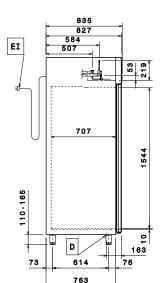
Electrical inlet (power) ΕI Refrigerant Inlet RO Refrigerant Outlet
